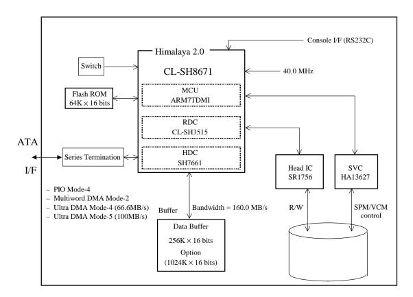
Figure 4.2 MPG3xxxAT Block diagram
